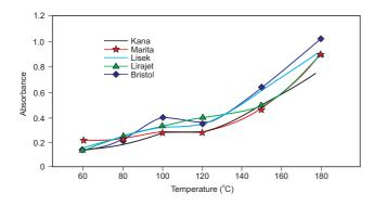
**Fig. 2.** Changes to the absorbance at 350 nm of oils in respect of changes to the drying temperature.
